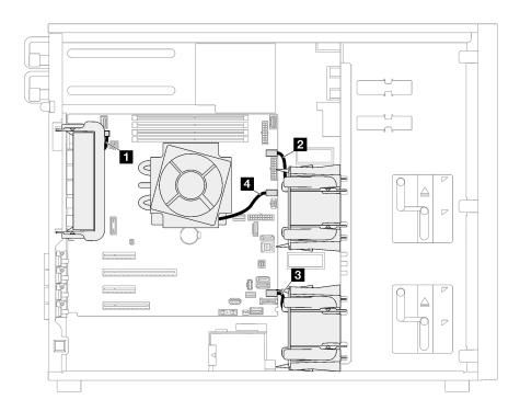
Figure 19. Fan power cable routing
