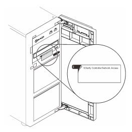
Figure 2. Location of XClarity Controller network access label
