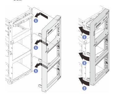
Figure 52. Installing the front bezel
