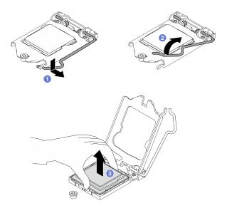
Figure 100. Opening the processor retainer
