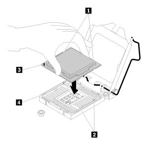
Figure 102. Installing the processor
