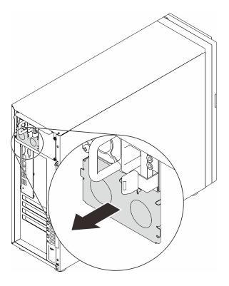
Figure 98. Removing a hot-swap power supply filler
