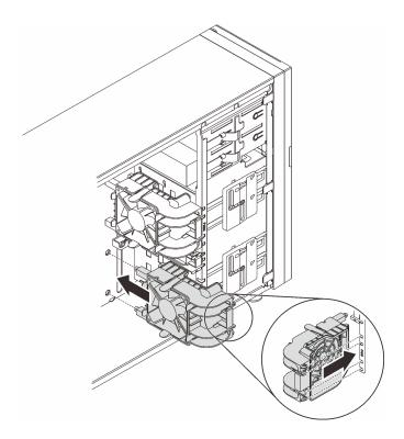
Figure 47. Installing the front system fan
