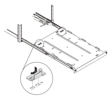
$\label{thm:continuous} Step \, 4. \quad \text{Install the four rubber safety pads as illustrated}.$
