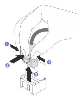
Remove the drive cage from the chassis (see "Remove the 3.5-inch/2.5-inch drive cage" on page Step 3. **64**).
