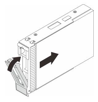
Figure 37. Installing the hot-swap drive
