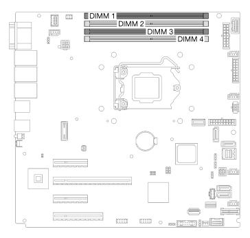
Figure 75. Memory module slots on the system board
