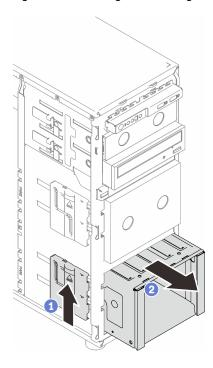
Remove the backplane or backplate (see "Remove the 3.5-inch/2.5-inch hot-swap drive backplane" on page 68 or "Remove the 3.5-inch simple-swap drive backplate" on page 71).
