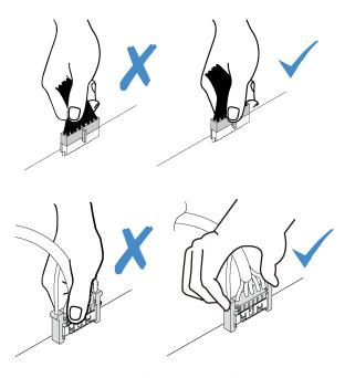
2. When installing the front system fan into the chassis, make sure the cables do not interfere with the two posts and the fan is firmly seated.
