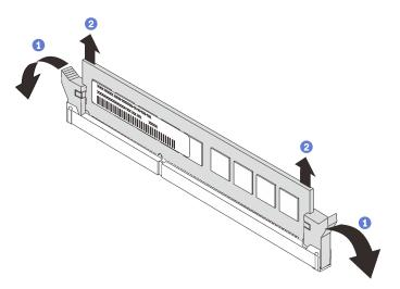
Figure 74. Removing a memory module
