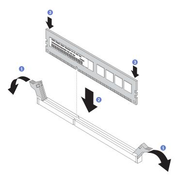
Figure 78. Installing a memory module
