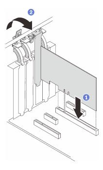
Figure 84. Installing a PCIe adapter
