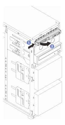
Figure 55. Removing the front panel board assembly
