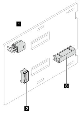
Figure 12. Power distribution board for hot-swap power supplies
