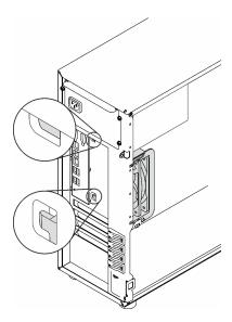
Figure 50. Installing the rear system fan
