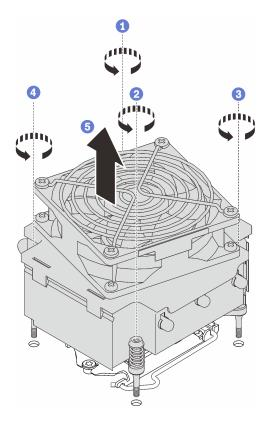
Figure 57. Removing the heat sink and fan module
