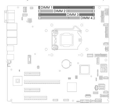
Figure 72. Memory module slots on the system board
