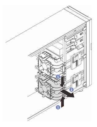
Figure 46. Removing the front system fan
