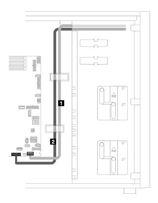
Figure 20. Cable routing for the front panel
