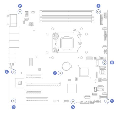
Figure 113. Tightening the screws to secure the system board
