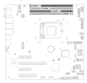
Figure 76. Memory module slots on the system board
