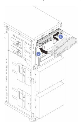
Figure 56. Installing the front panel board assembly
