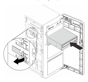
Figure 82. Installing an optical drive
