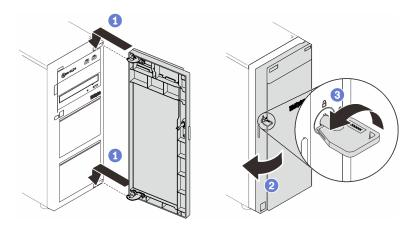
Figure 54. Installing the front door
