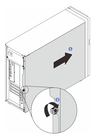
Figure 110. Securing the server cover to the chassis
