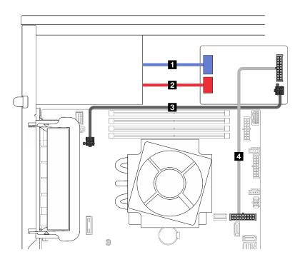
Figure 21. Cable routing for the fixed power supply
