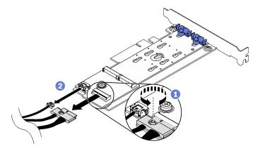
Figure 62. Disconnecting the power and signal cables
