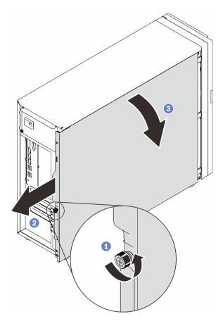
Figure 108. Removing the server cover
