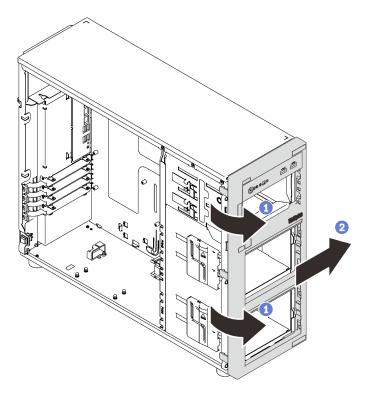
Figure 51. Removing the front bezel
