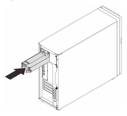
Figure 99. Installing a hot-swap power supply
