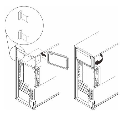
Figure 93. Installing a fixed power supply bracket
