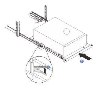
Step 8. Secure the tray with two M6 x 16 screws to the front of the rack cabinet.
