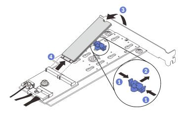
Figure 68. Removing an M.2 drive
