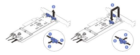
Figure 69. Adjusting the M.2 retainer
