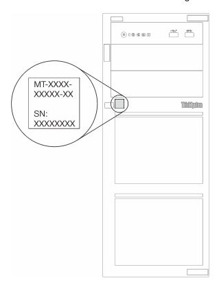
Figure 1. Location of the machine type, model, and serial number
