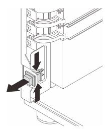
Figure 59. Removing the intrusion switch
