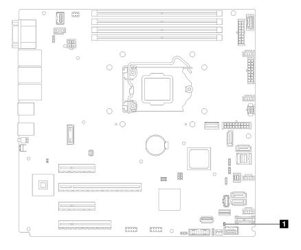
Figure 9. System-board LED
