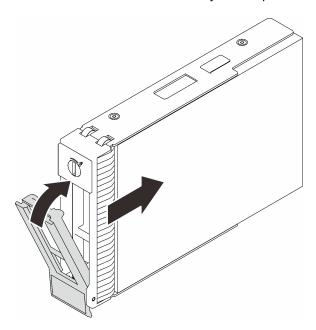
Figure 40. Installing the simple-swap drive
