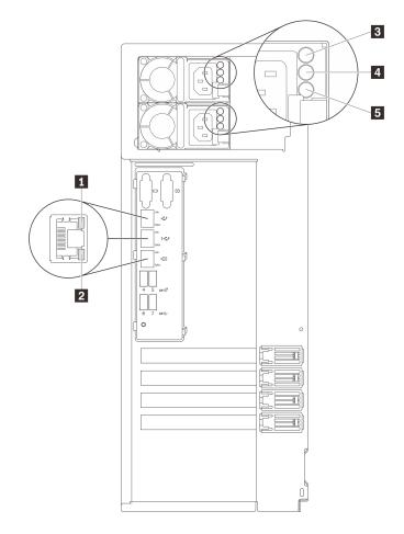
Figure 7. Rear view LEDs of the server
