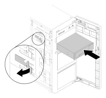
Figure 115. Installing a tape drive
