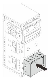
Figure 26. Installing the drive cage
