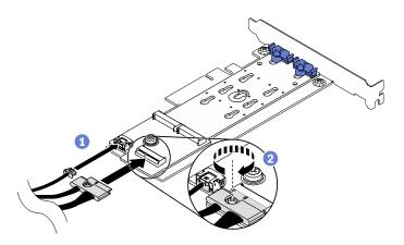
Figure 66. Installing the M.2 power and signal cables
