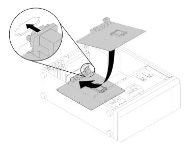
Figure 112. Installing the system board
