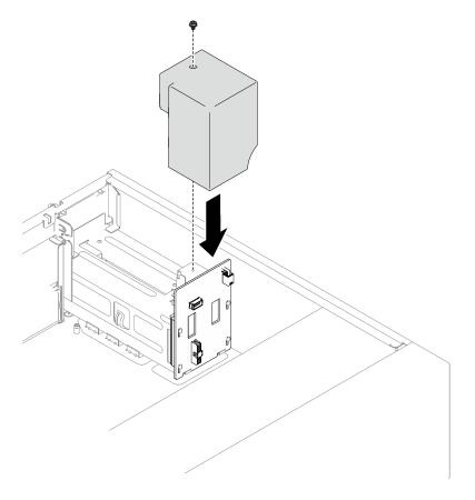
Figure 89. Installing the power distribution board cover
