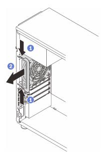
Figure 48. Removing the rear system fan
