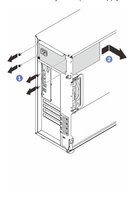
Figure 91. Removing a fixed power supply
