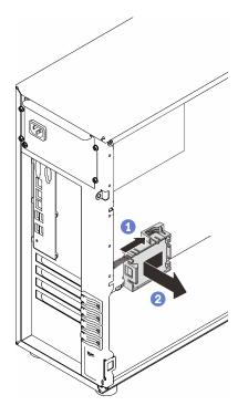
Figure 104. Removing the RAID flash power module and bracket assembly from the chassis
