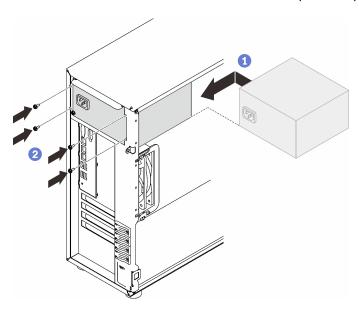
Figure 94. Installing a fixed power supply
