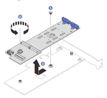
Figure 63. Removing the M.2 boot adapter
