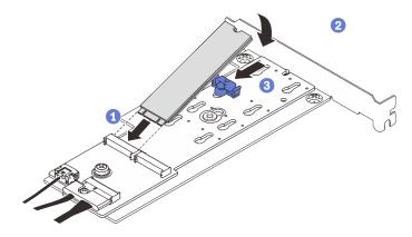
Figure 71. Installing an M.2 drive
