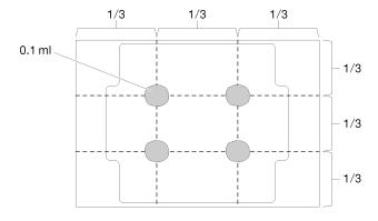
Figure 101. Proper shape of the thermal grease
