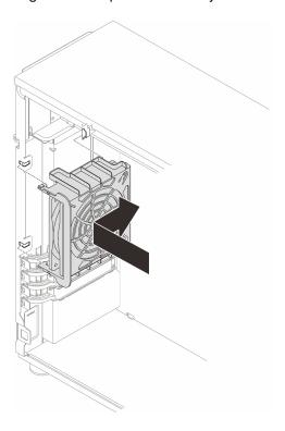
Figure 49. Positioning the rear system fan into the chassis
