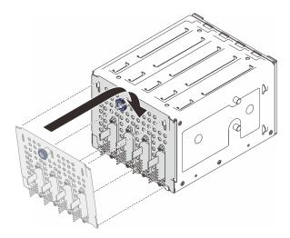
Figure 32. Installing the simple-swap drive backplate
