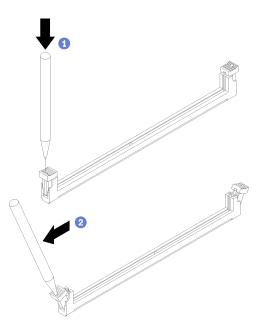
Figure 73. Opening retaining clips
