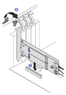
Figure 67. Installing the PCIe adapter into the chassis
