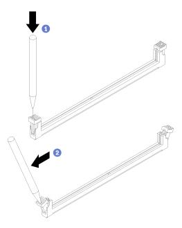
Figure 77. Opening retaining clips
