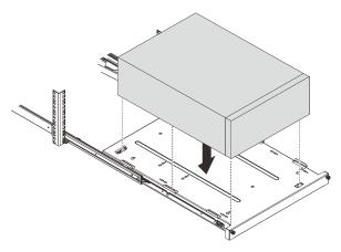
Step 7. Install the server into the rack cabinet.
