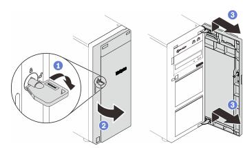
Figure 53. Removing the front door
