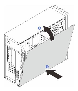
Figure 109. Positioning the server cover onto the chassis
