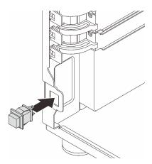
Figure 60. Installing the intrusion switch
