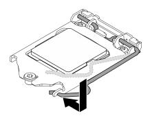
Figure 103. Closing the processor retainer
