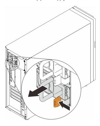
Figure 96. Removing a hot-swap power supply
