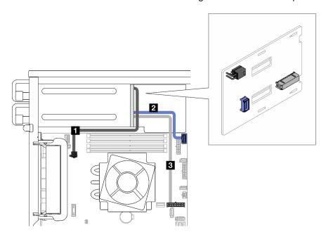
Figure 22. Cable routing for the redundant power supplies
