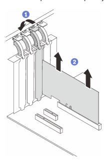
Figure 83. Removing a PCIe adapter
